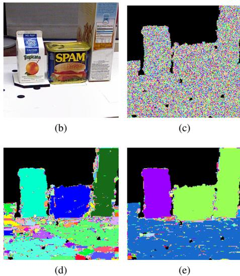
Fig. 7: (a) Frequency of correct pose estimates as a function of the granularity of the segmentation. Finer segmentation occurs for smaller values of the angular threshold. (b) Example frame from the dataset. (c)-(e) Segmentations for thresholds of  $0^\circ$ ,  $8^\circ$ , and  $12^\circ$  respectively. Note the under-segmentation in (e).
