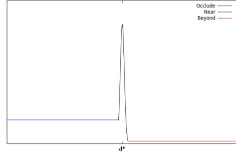
Fig. 2: Piecewise sensor model used in IBM. On the x-axis is the beam measurement  $d_i$ .  $d_i^*$  is the expected measurement from the model. Not to scale.
