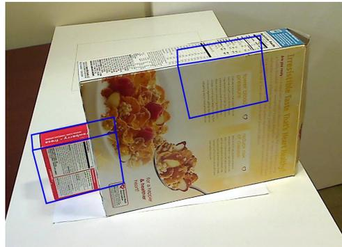
Fig. 1: Scene with clutter and occlusion. Matching the small box based on its 3D model is problematic. ICP will match the model with free-space protrusions, as on the occluded box at left. The beam model will find the correct match there, but will prefer to embed the smaller box model into the larger box, where the whole front surface matches.
